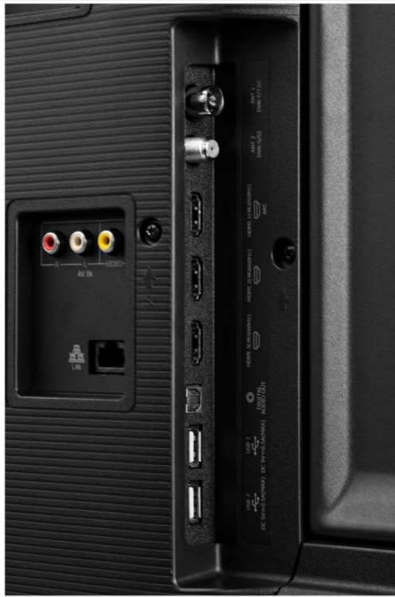
Figure 3: Rear view of the Hisense TV's connectivity ports. This image displays the various input and output ports on the back of the television, including HDMI, USB, LAN, antenna, and AV inputs.
