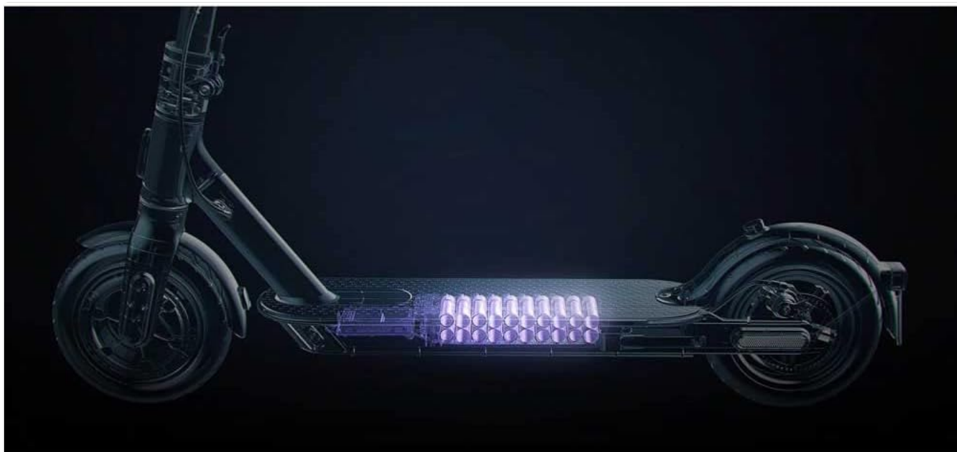
Figure 3: An illustrative cross-section revealing the internal lithium-ion battery cells housed within the scooter's deck, providing its power source.
