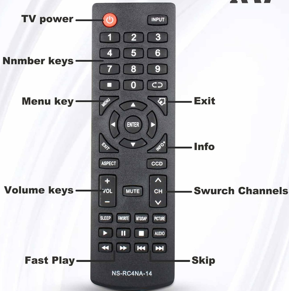
Figure 2: Remote Control Button Layout. This image illustrates the front of the remote control, highlighting and labeling key buttons such as TV power, number keys, menu, exit, info, volume, channel, fast play, and skip.
