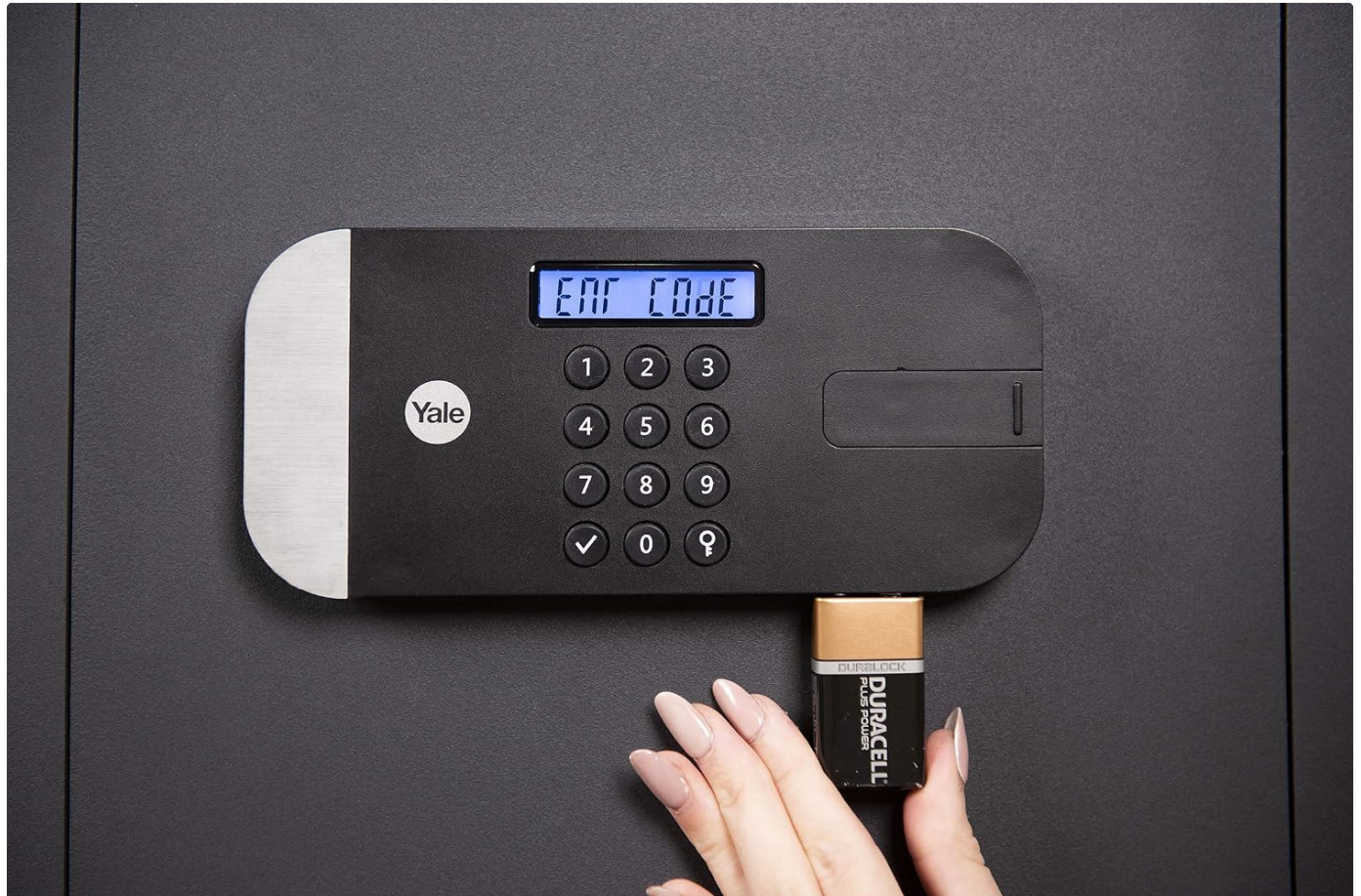
Image 6.1: A hand connecting a 9V battery to the external emergency power port on the safe's keypad, allowing temporary power for code entry.
