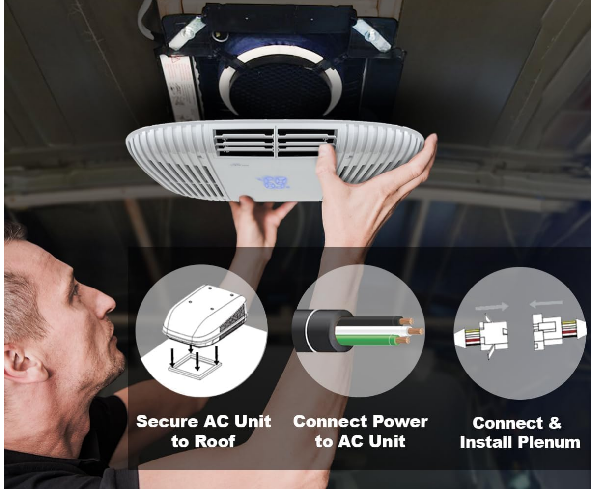
Figure 3.3: Visual guide to the three main steps for installing the RecPro RV Air Conditioner.
