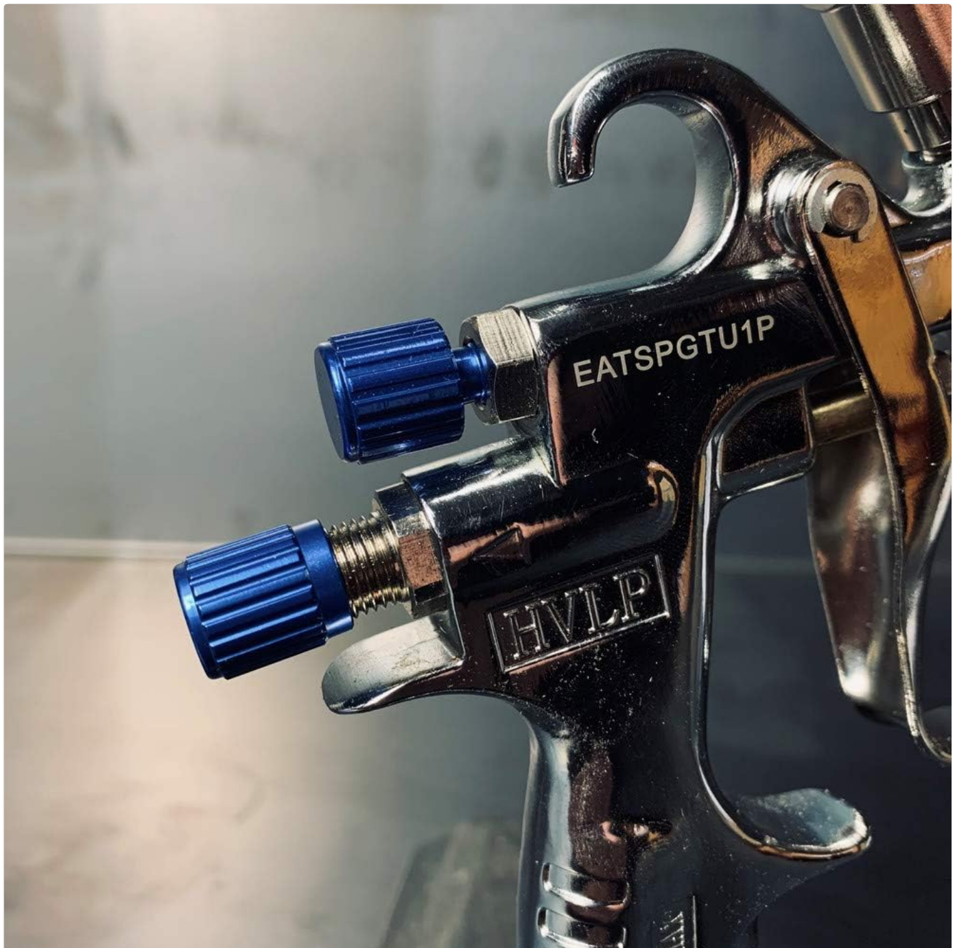
Figure 3: Close-up of the spray gun's adjustment knobs for air and fluid control.
