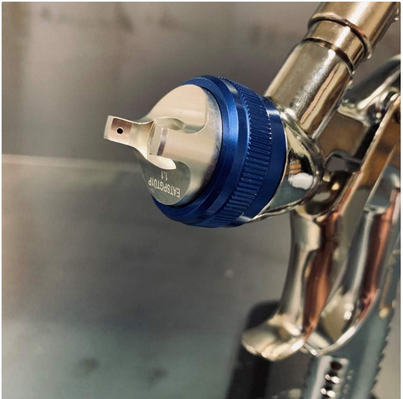
Figure 4: Detail of the spray gun's 1.1mm tip, indicating precision for touch-up work.
