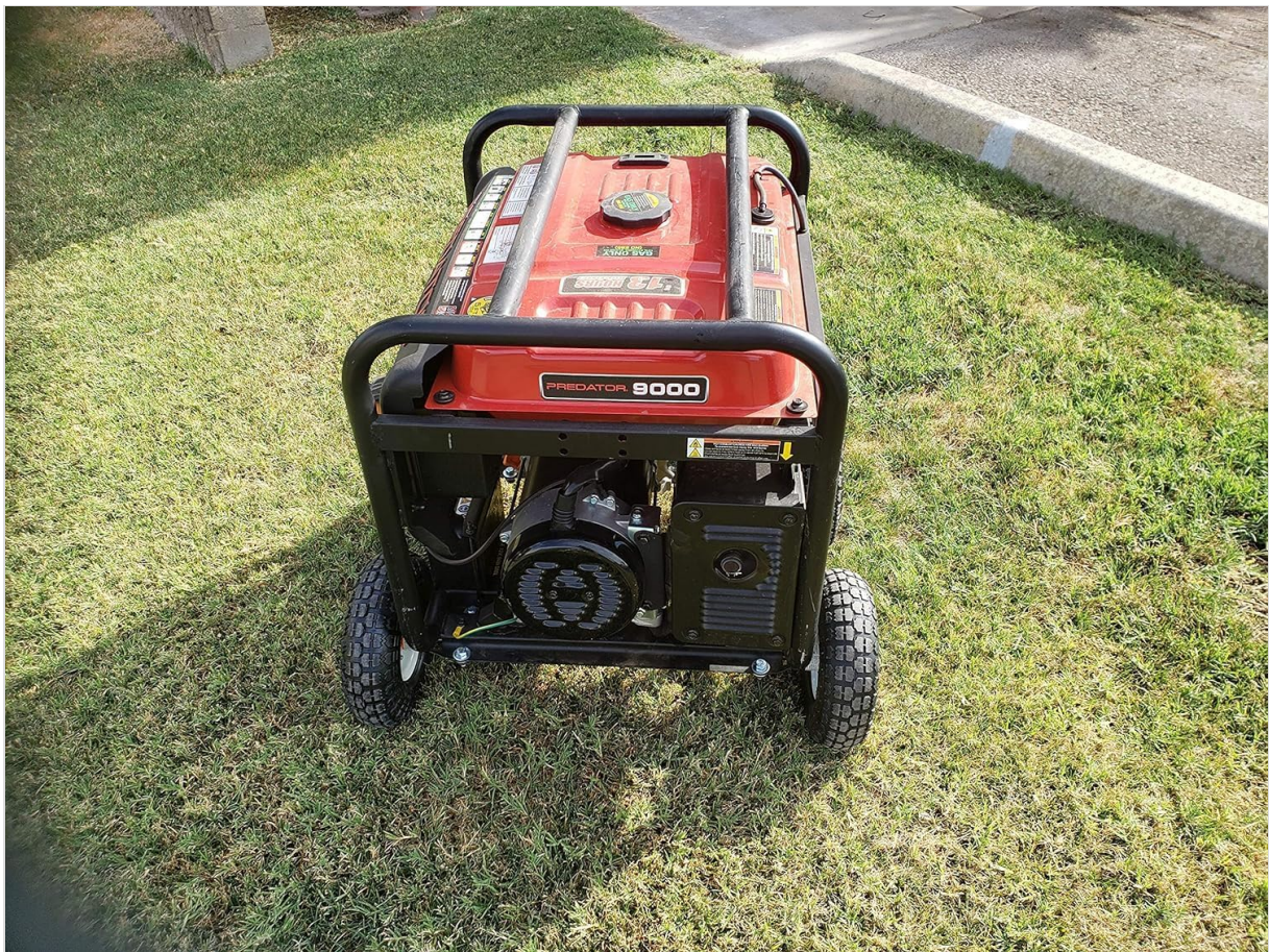
Image 1: Top-down view of a Predator generator with the wheel kit successfully installed, showing the four wheels and axle assemblies.
