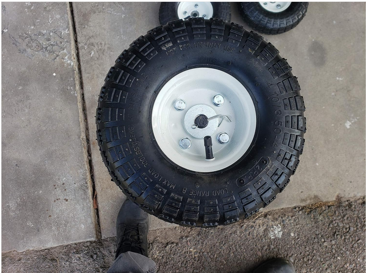
Image 3: Detailed view of one of the 10-inch inflatable wheels, showing the cotter pin mechanism that secures it to the axle shaft.
