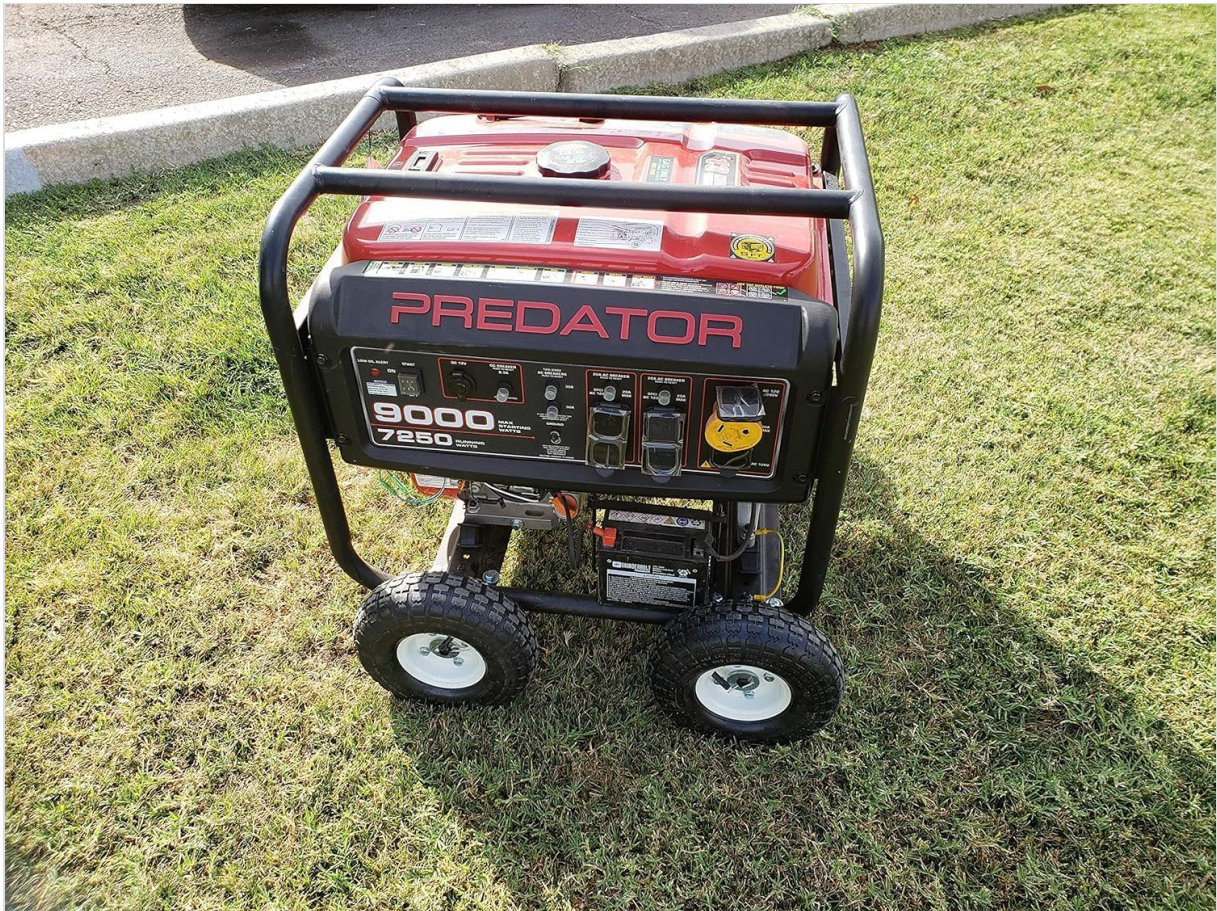
Image 2: Front view of the Predator generator equipped with the wheel kit, demonstrating the added ground clearance and stability.
