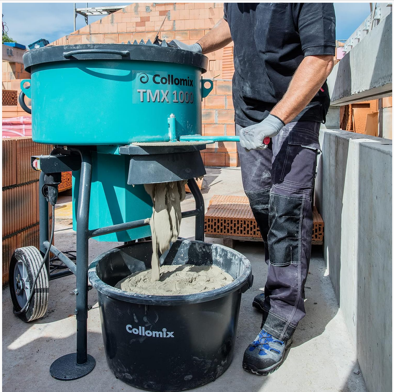
Figure 5: The TMX1000 mixer discharging freshly mixed material into a bucket.
