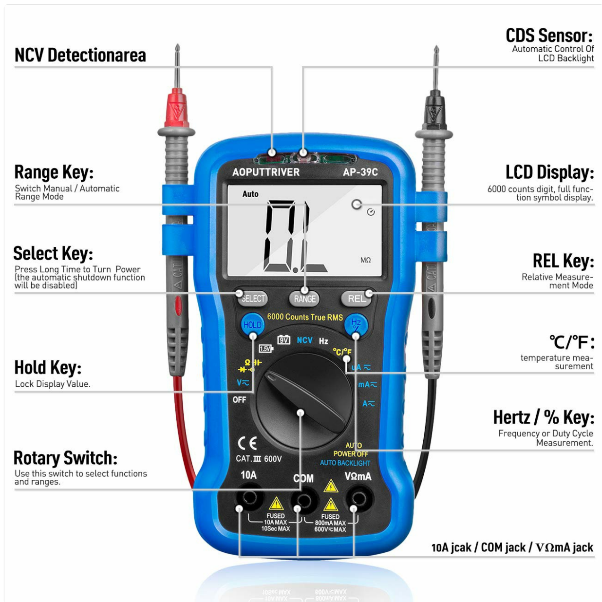
Figure 3.1: Front view of the AOPUTTRIVER AP-39C Digital Multimeter with key components labeled. This includes the LCD display, function buttons (SELECT, RANGE, REL, HOLD), rotary switch, NCV detection area, and input jacks.
