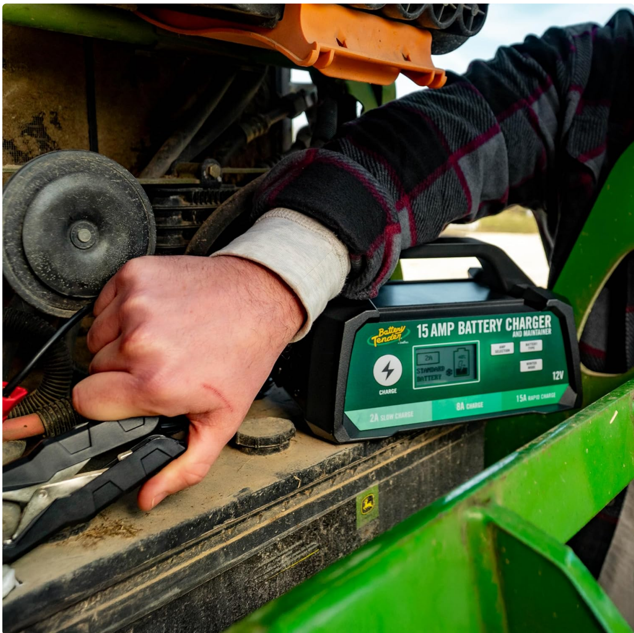
Figure 3: Proper connection of the Battery Tender charger to a vehicle battery, showing the red clamp on the positive terminal and the black clamp on the negative terminal.
