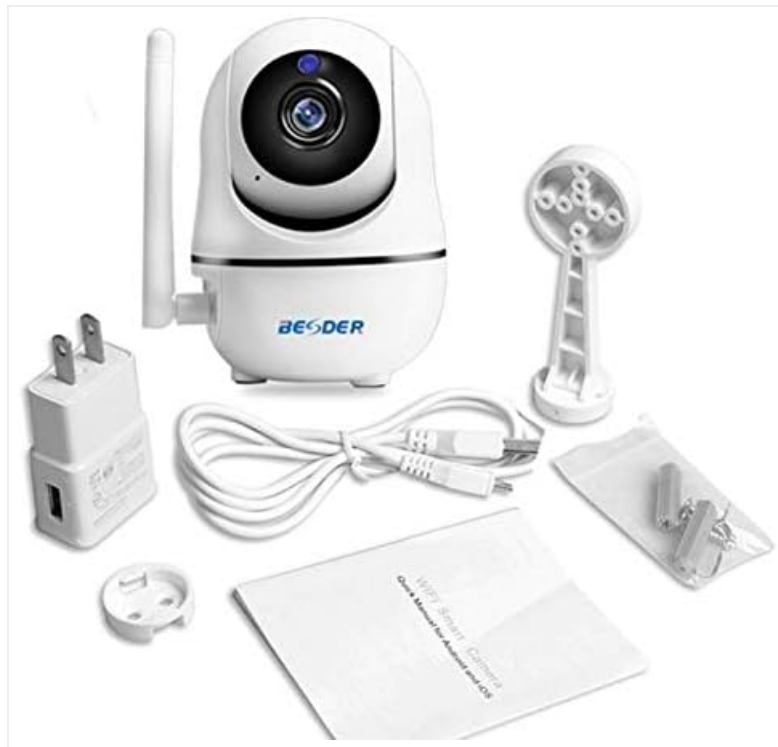
Figure 1: Package contents of the BESDER Smart Home Security Camera, showing the camera unit, power adapter, USB cable, mounting bracket, screws, and the user manual.
