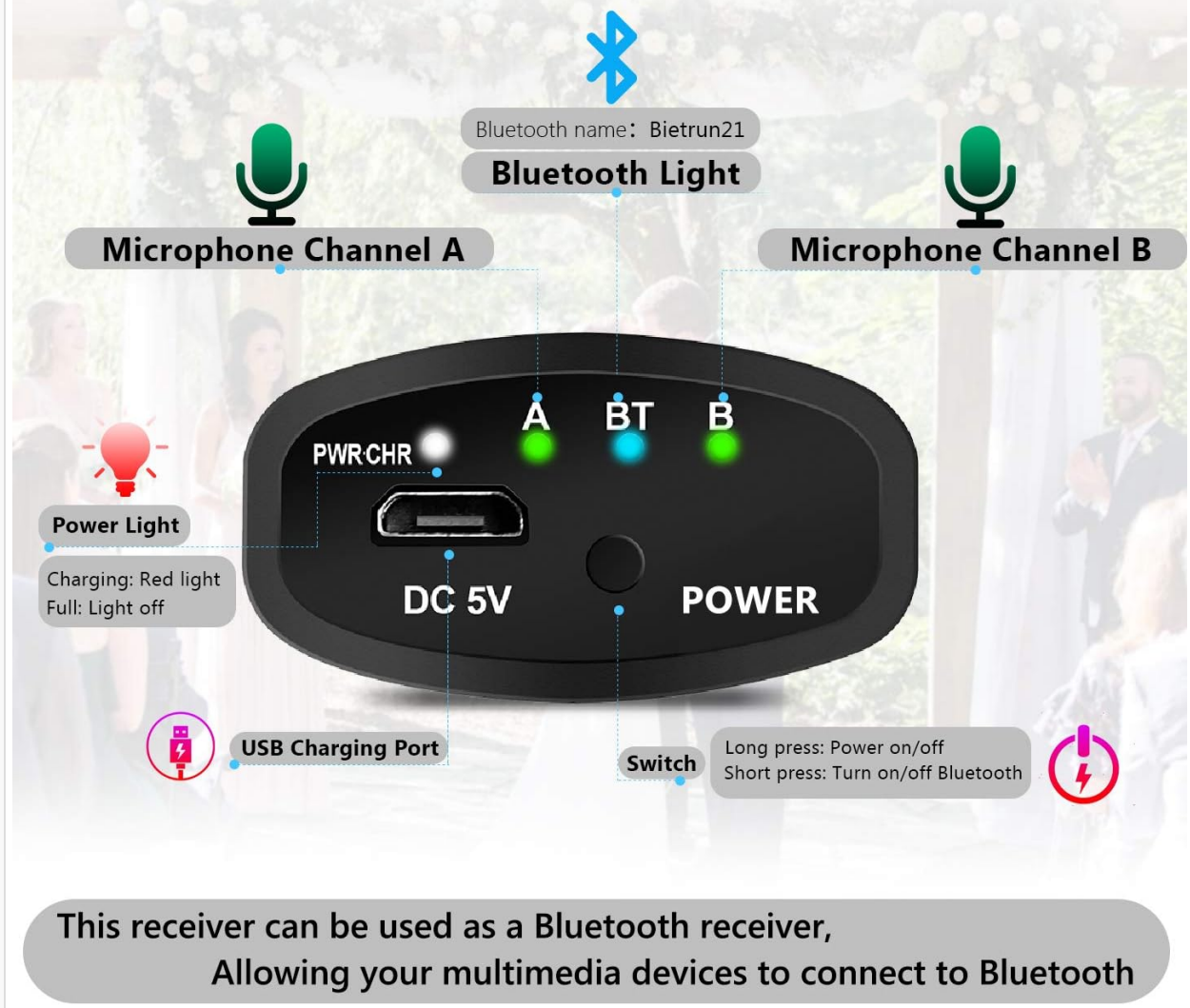
Figure 3.2: Receiver Charging and Indicators. Details the USB charging port, power light (red for charging, off when full), and lights for Microphone Channel A, Bluetooth, and Microphone Channel B.
