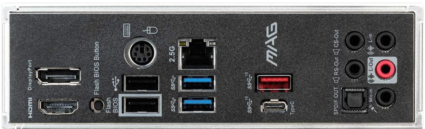
Figure 2.4: Rear I/O panel of the motherboard, detailing the various ports including USB, HDMI, DisplayPort, and LAN.
