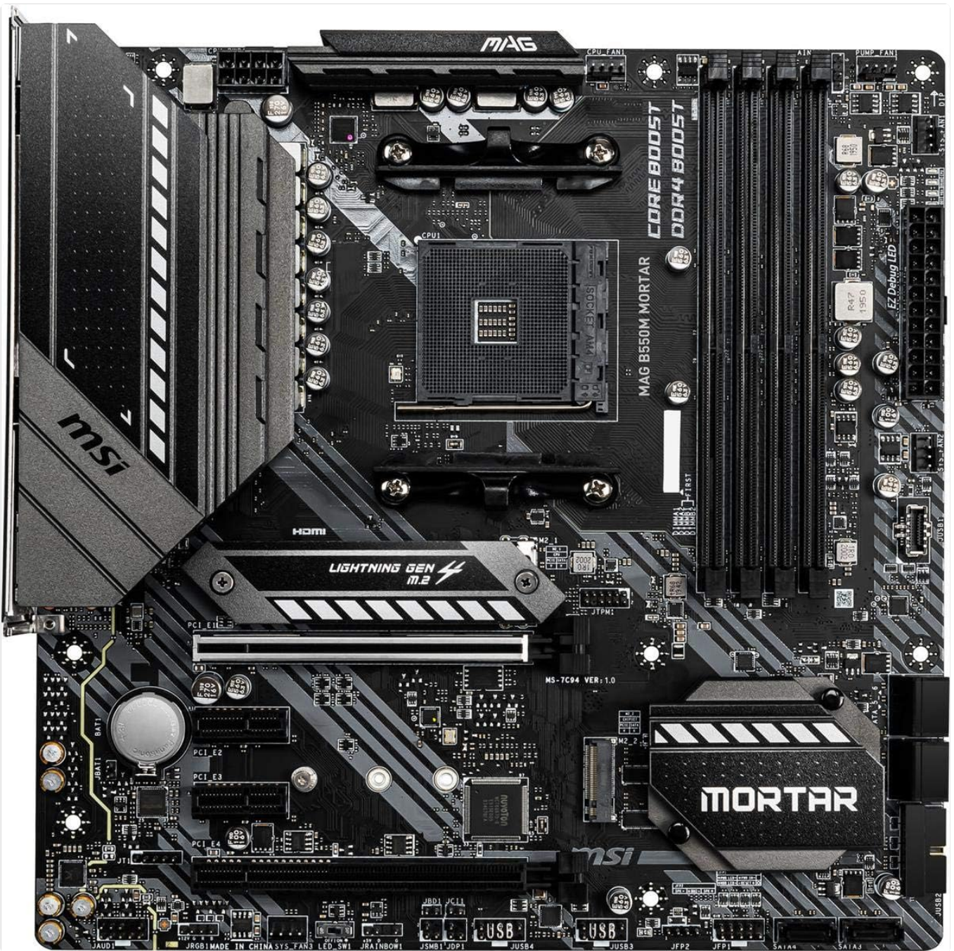
Figure 2.2: Top-down view of the motherboard, showing the CPU socket, RAM slots, and PCIe slots.
