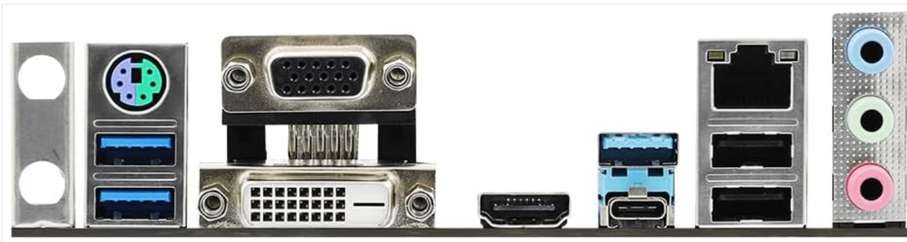
Image 2: Rear I/O panel of the ASRock Z390 Phantom Gaming 4-1B motherboard, showing various connectivity ports.
