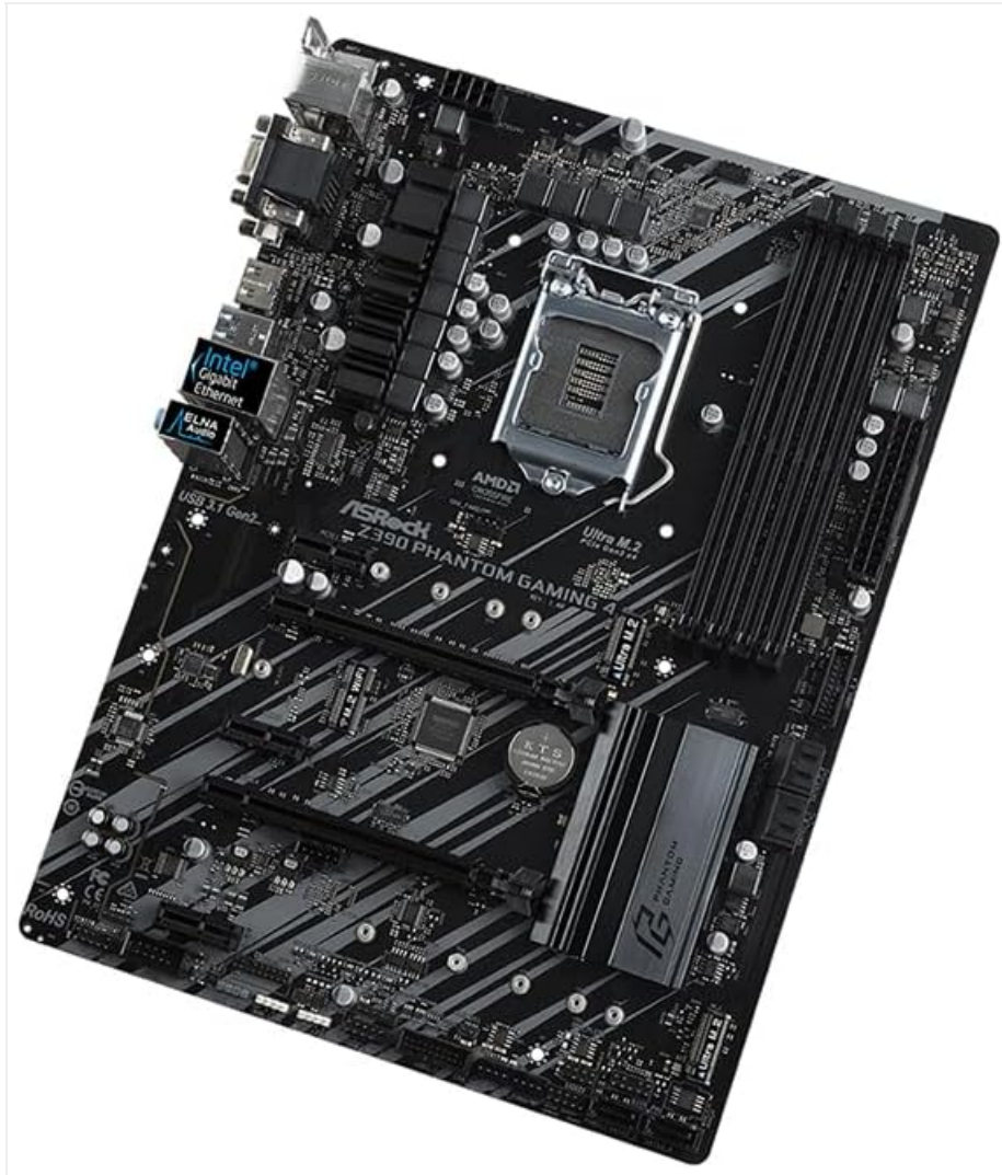
Image 1: Top view of the ASRock Z390 Phantom Gaming 4-IB motherboard, showing the CPU socket, RAM slots, PCIe slots, and various headers.
