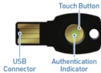
Image 3.1: Diagram illustrating the USB Connector, Touch Button, and Authentication Indicator on the FeiTian A4B USB Security Key.
