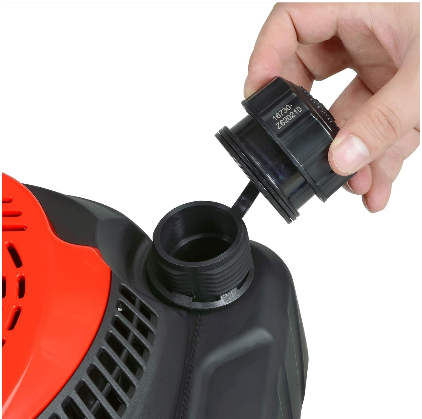
Image: Opening the fuel cap to add gasoline. Always ensure the engine is off and cool before refueling.
