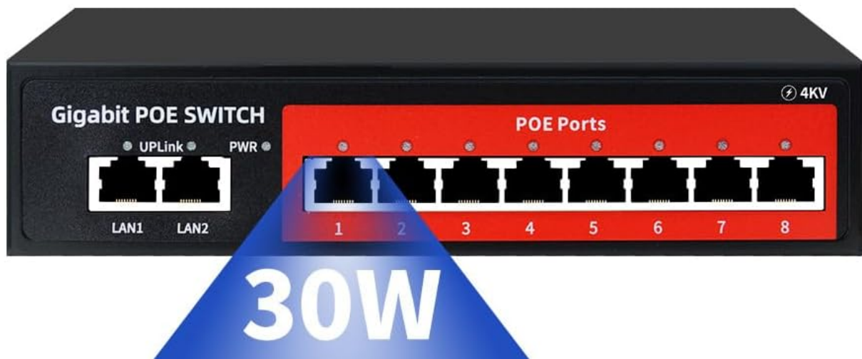
Figure 4.2: Close-up of the switch ports, highlighting the 2 Gigabit Uplink ports (LAN1, LAN2) and 8 Gigabit PoE ports (1-8). The AI PWR switch is also visible.
