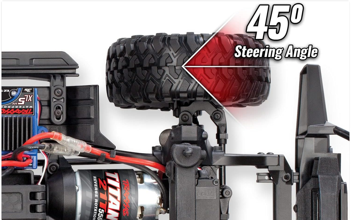
Figure 4.1: Illustration of the 45-degree steering angle for enhanced maneuverability.
