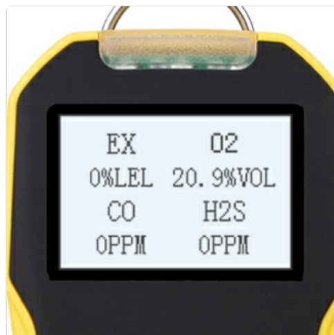
Figure 3.2: Close-up of the LCD panel, displaying gas concentrations and device status.
