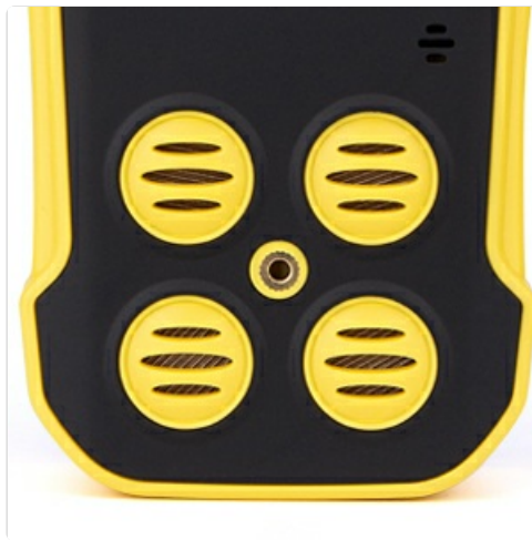
Figure 3.4: The gas detection sensor hole, where ambient air is drawn in for analysis.
