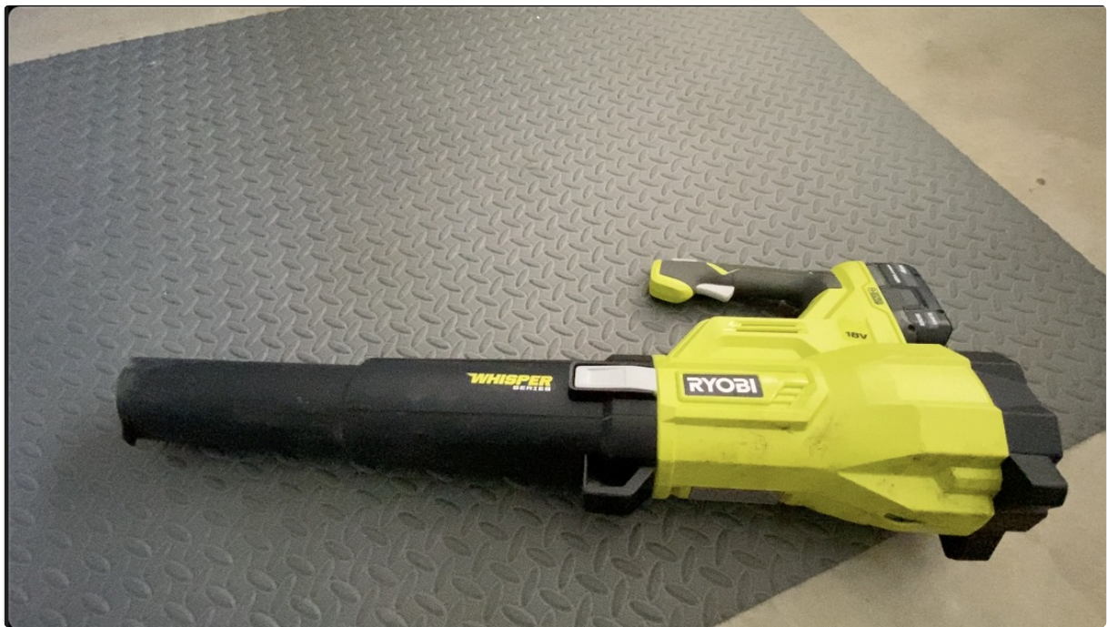
Image: RYOBI P21010BTLVNM Blower with an 18V battery pack inserted into the top slot. The battery has a charge indicator visible.
