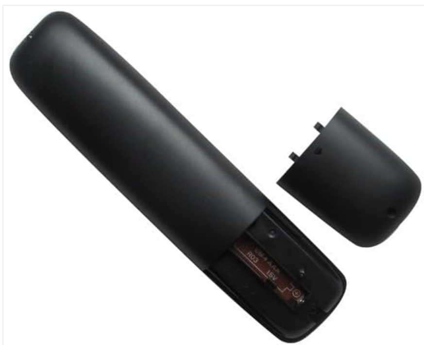
Figure 2.2: The remote control with the battery compartment open, illustrating the correct orientation for AAA battery insertion.
