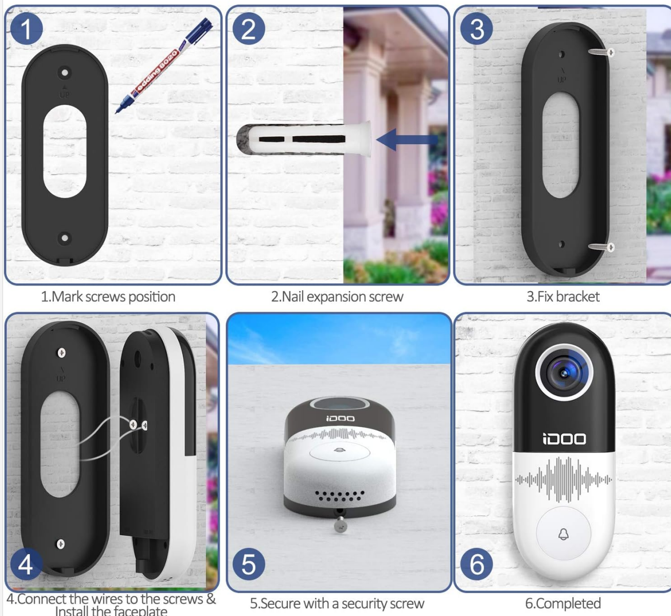
Figure 3: Step-by-Step Installation Process. This visual guide demonstrates the six key steps for installing the iDOO Video Doorbell: 1. Marking screw positions, 2. Inserting expansion screws, 3. Fixing the bracket, 4. Connecting wires and installing the faceplate, 5. Securing with a security screw, and 6. Completing the installation.
