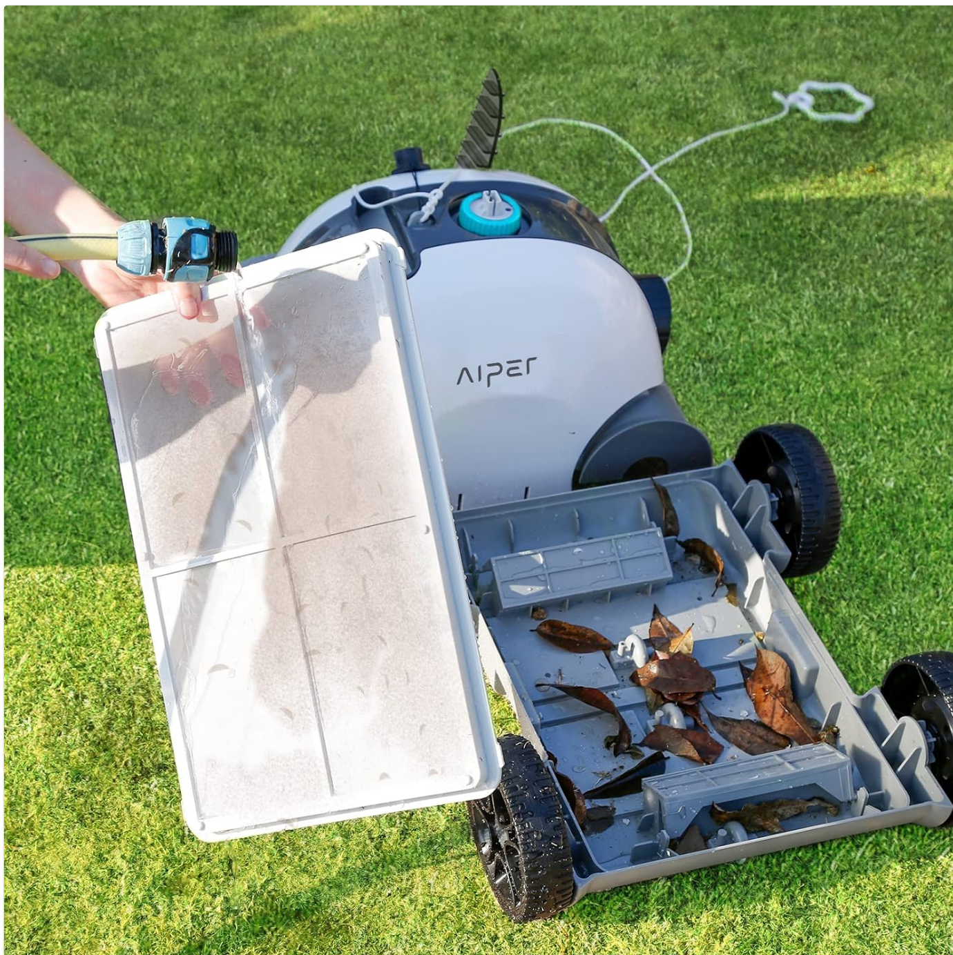
Figure 8: Cleaning the filter basket after use.
