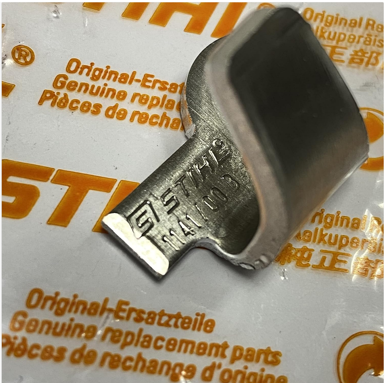
Figure 3: Close-up of the Stihl Chain Catcher, displaying the engraved OEM part number 1141 656 7700. This detail confirms the authenticity and specific model of the part.
