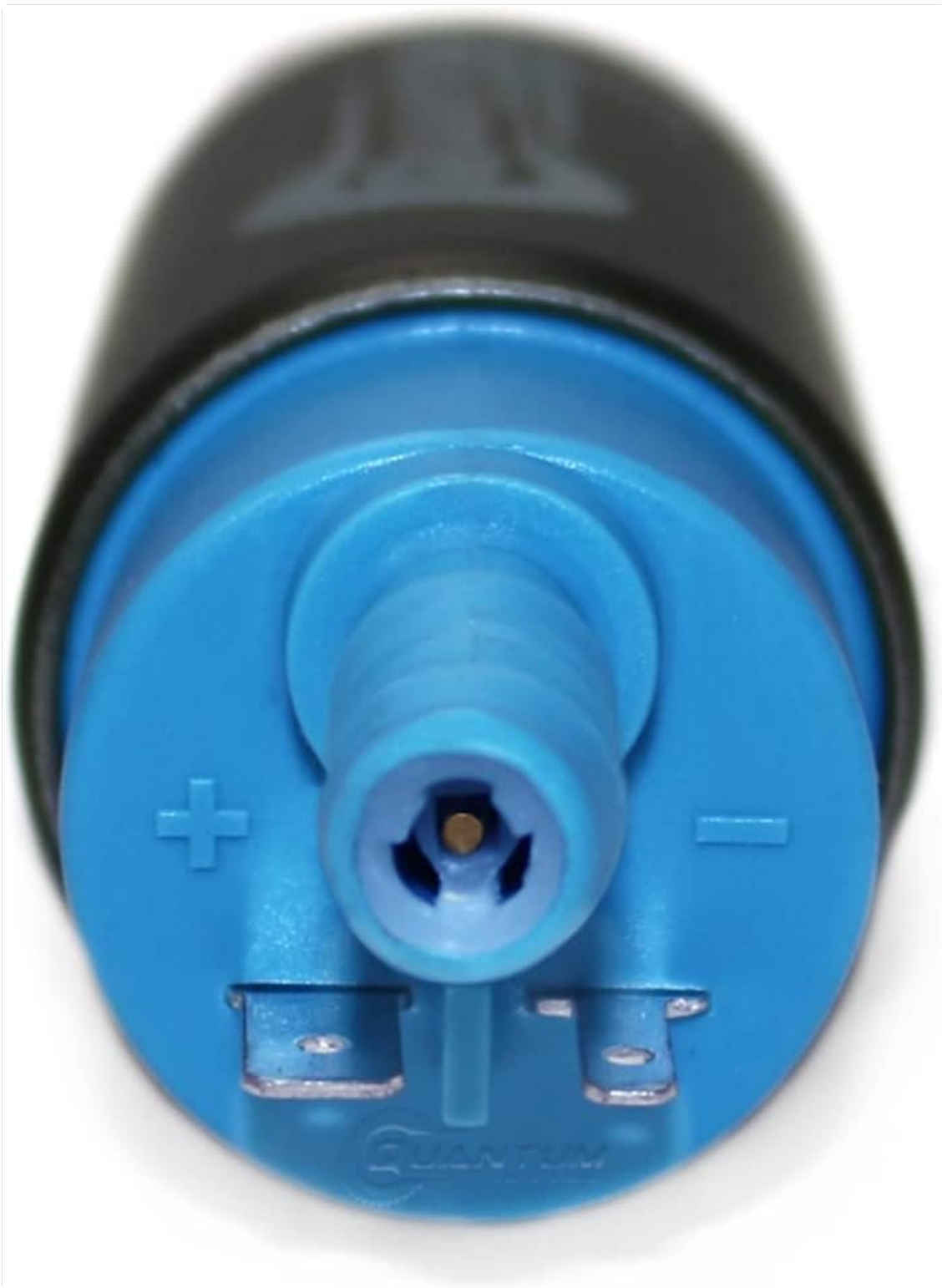
Figure 2: Fuel Pump (Electrical Connector End)
