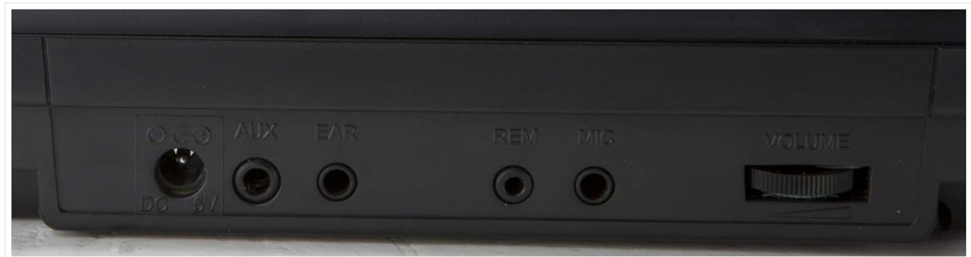
Figure 2: Side Panel Ports. This image shows the side panel of the onn Cassette Recorder, highlighting various input and output ports. From left to right, these include a 'DC 6V' power input, 'AUX' input, 'EAR' (earphone/headphone) output, 'REM' (remote) input, 'MIC' (external microphone) input, and a 'VOLUME' control dial.
