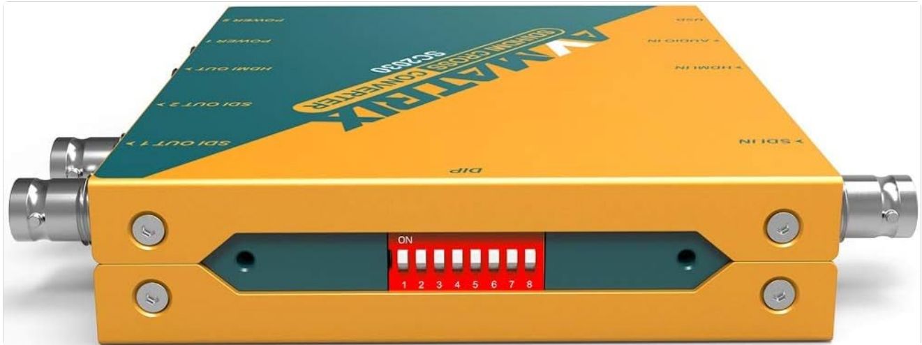
Figure 3.2: Side view of the SC2030 Converter highlighting the DIP switches for configuration.
