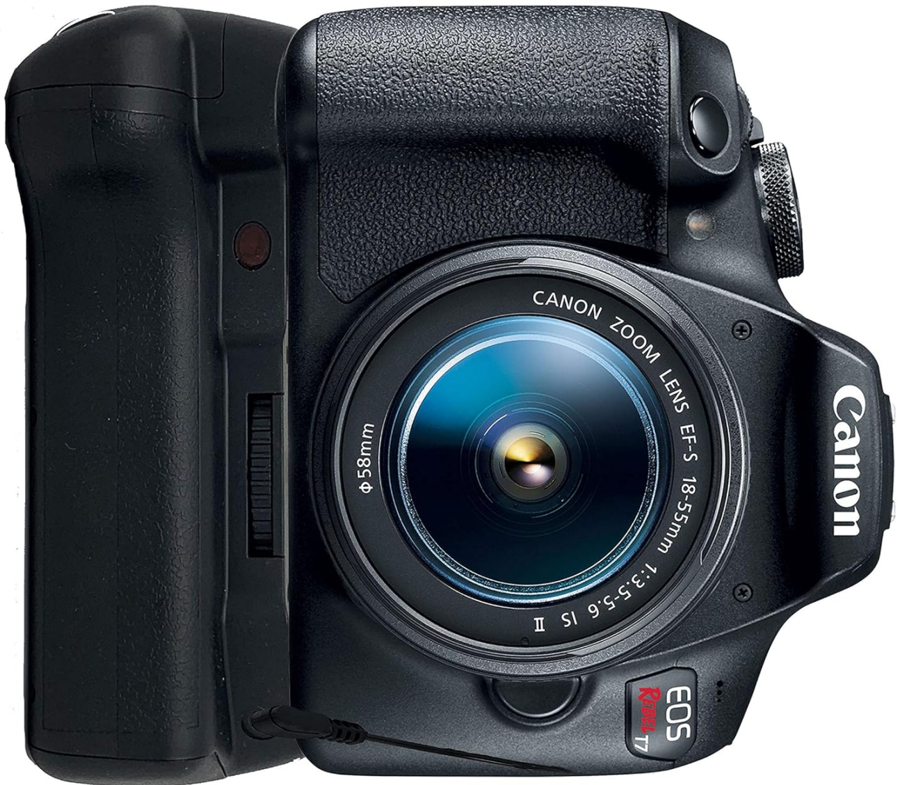
Figure 4.1: Camera with battery grip attached, demonstrating its use for portrait orientation photography.
