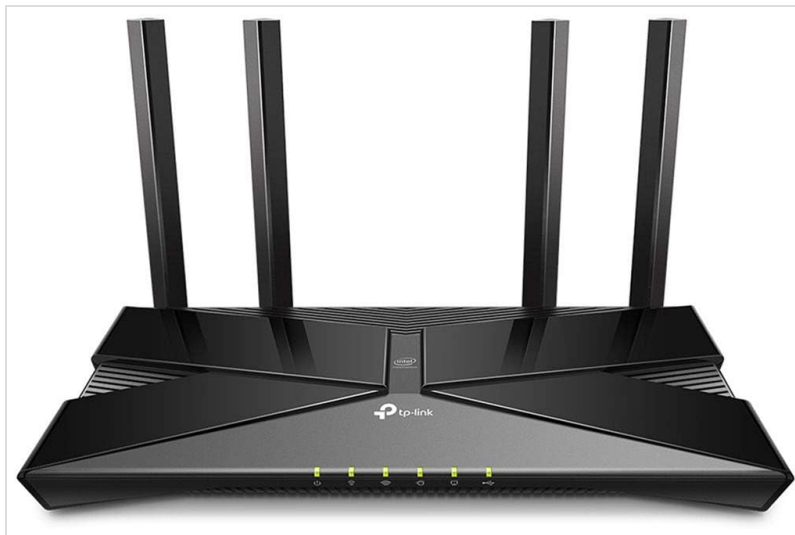
Figure 3.1: Front view of the TP-Link Archer AX50 AX3000 Wireless Dual-Band Gigabit Router, showcasing its four external antennas and front-facing LED indicators.
