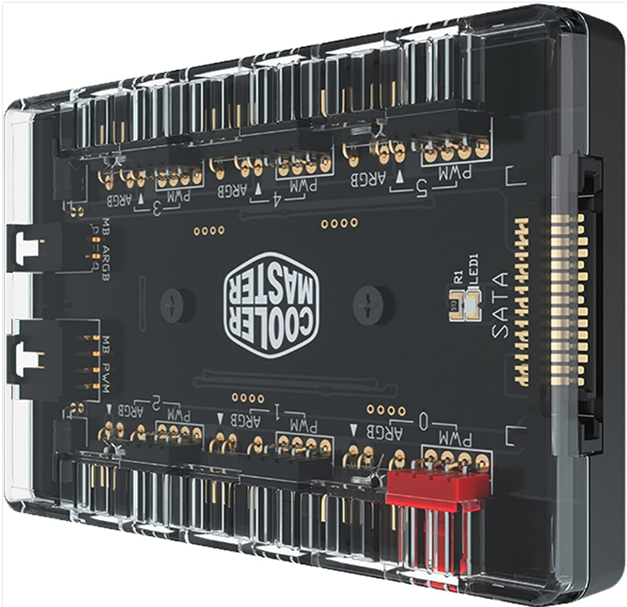
Image 2: Angled view of the hub, highlighting the SATA power input connector on the side.
