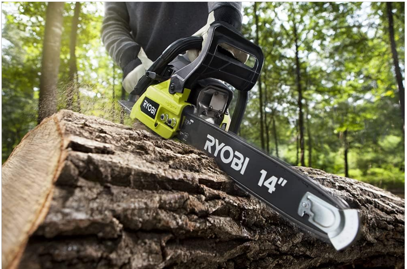
Figure 4.1: Proper operation of the Ryobi RY3714 chainsaw for cutting a log, demonstrating safe posture and grip.
