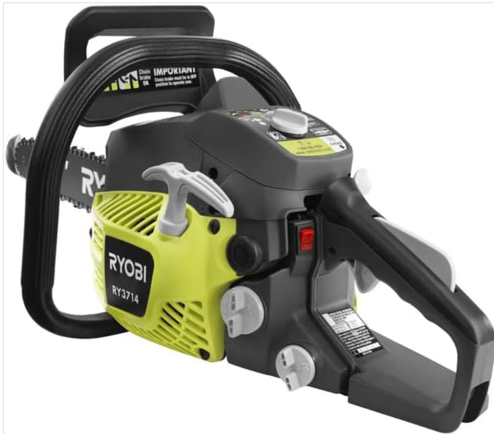
Figure 2.4: Close-up view of the Ryobi RY3714 14-inch Gas Chainsaw's control panel, showing the choke, primer bulb, and on/off switch.
