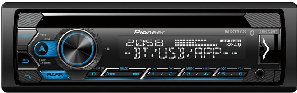
Figure 5.1: Front panel of the Pioneer DEH-S4250BT receiver, displaying the main display, rotary volume knob, source selection buttons, and various playback controls.
