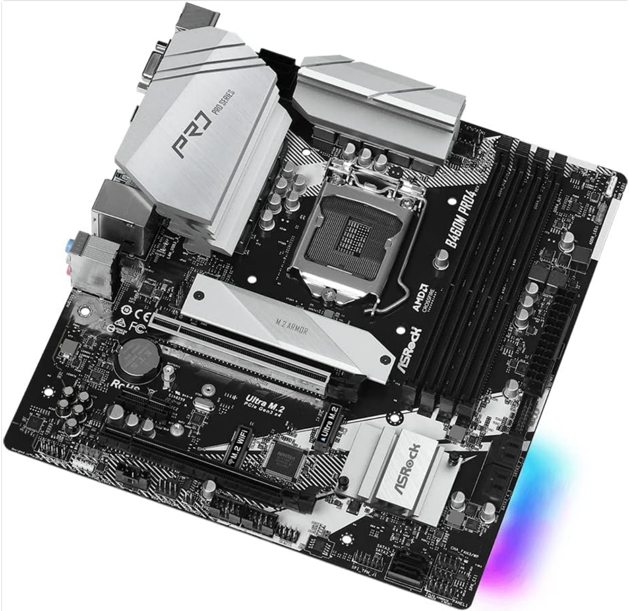
Image 3.2: Angled view of the ASRock B460M PRO4 Motherboard, illustrating the M.2 slots and SATA ports for storage devices.
