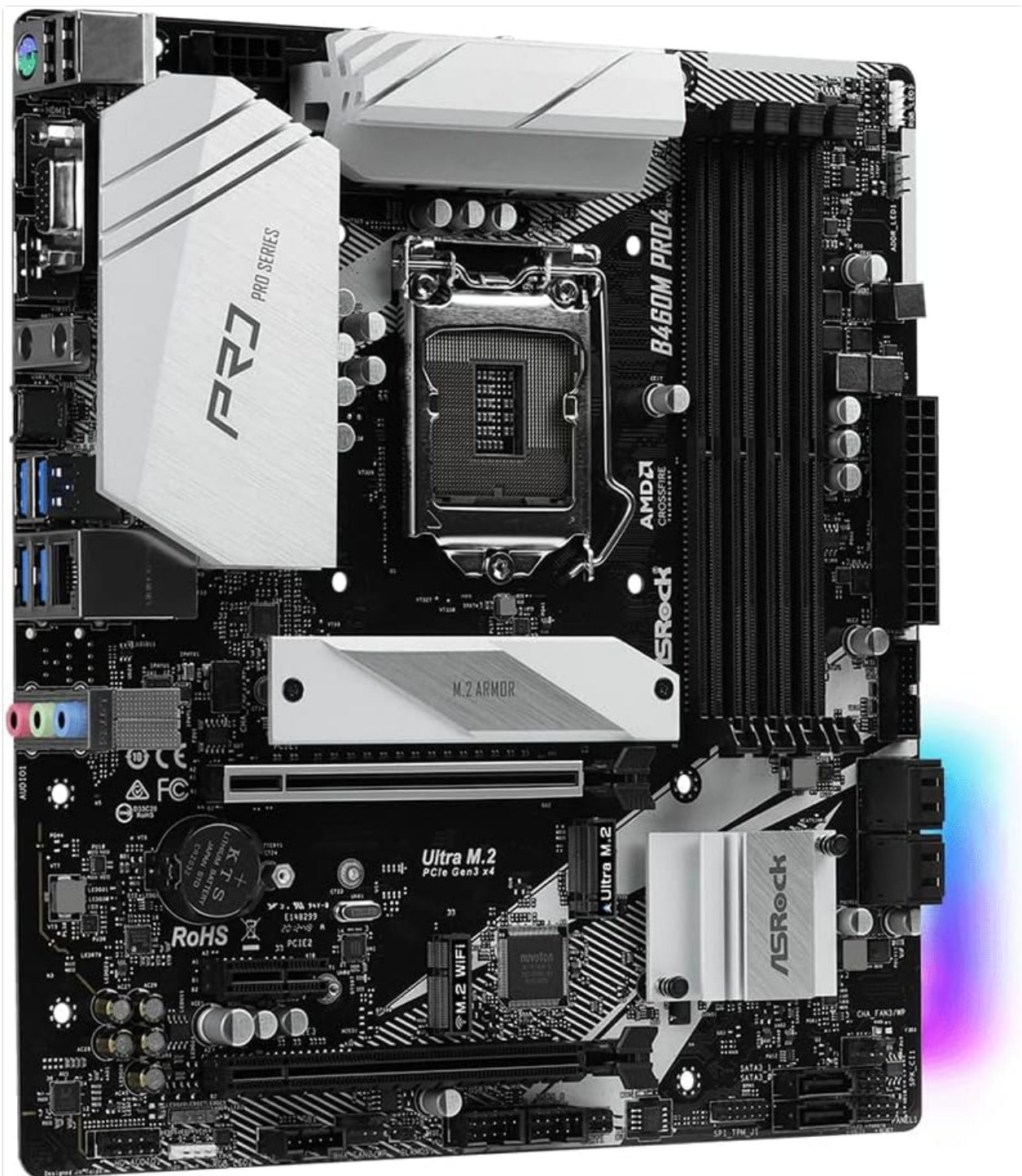
Image 3.3: ASRock B460M PRO4 Motherboard, showcasing the various PCIe expansion slots.
