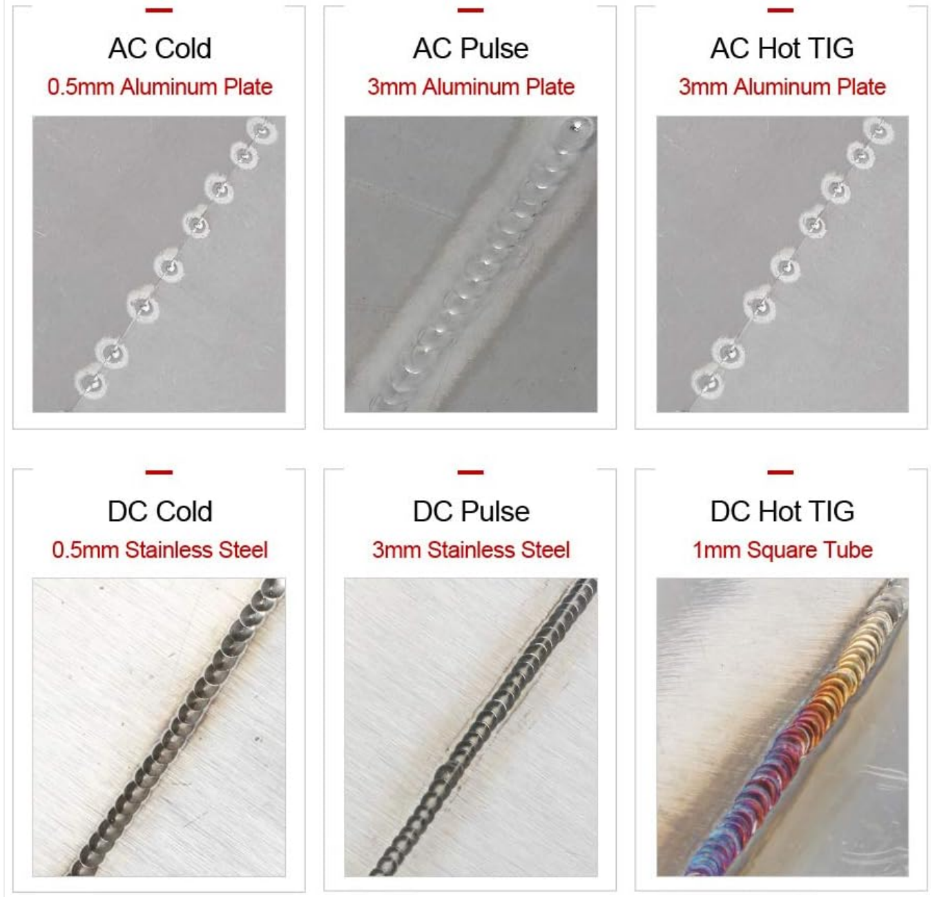
Figure 7: Examples of welding results for AC Cold (0.5mm Aluminum), AC Pulse (3mm Aluminum), AC Hot TIG (3mm Aluminum), DC Cold (0.5mm Stainless Steel), DC Pulse (3mm Stainless Steel), and DC Hot TIG (1mm Square Tube).
