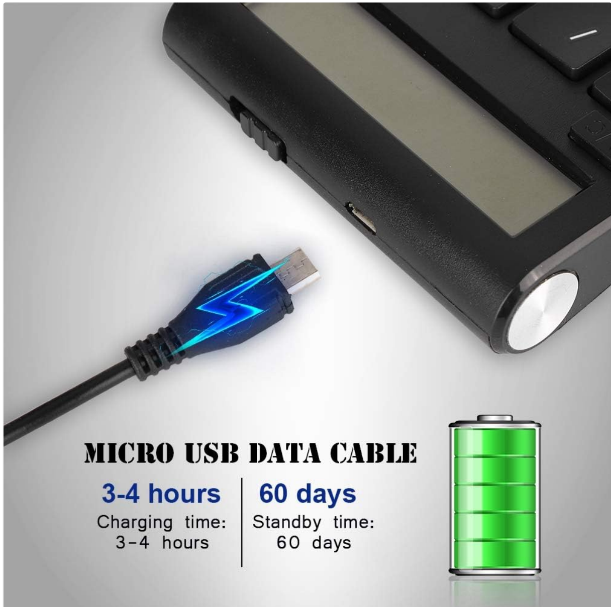
Figure 6.1: Charging the keypad with the Micro USB cable.
