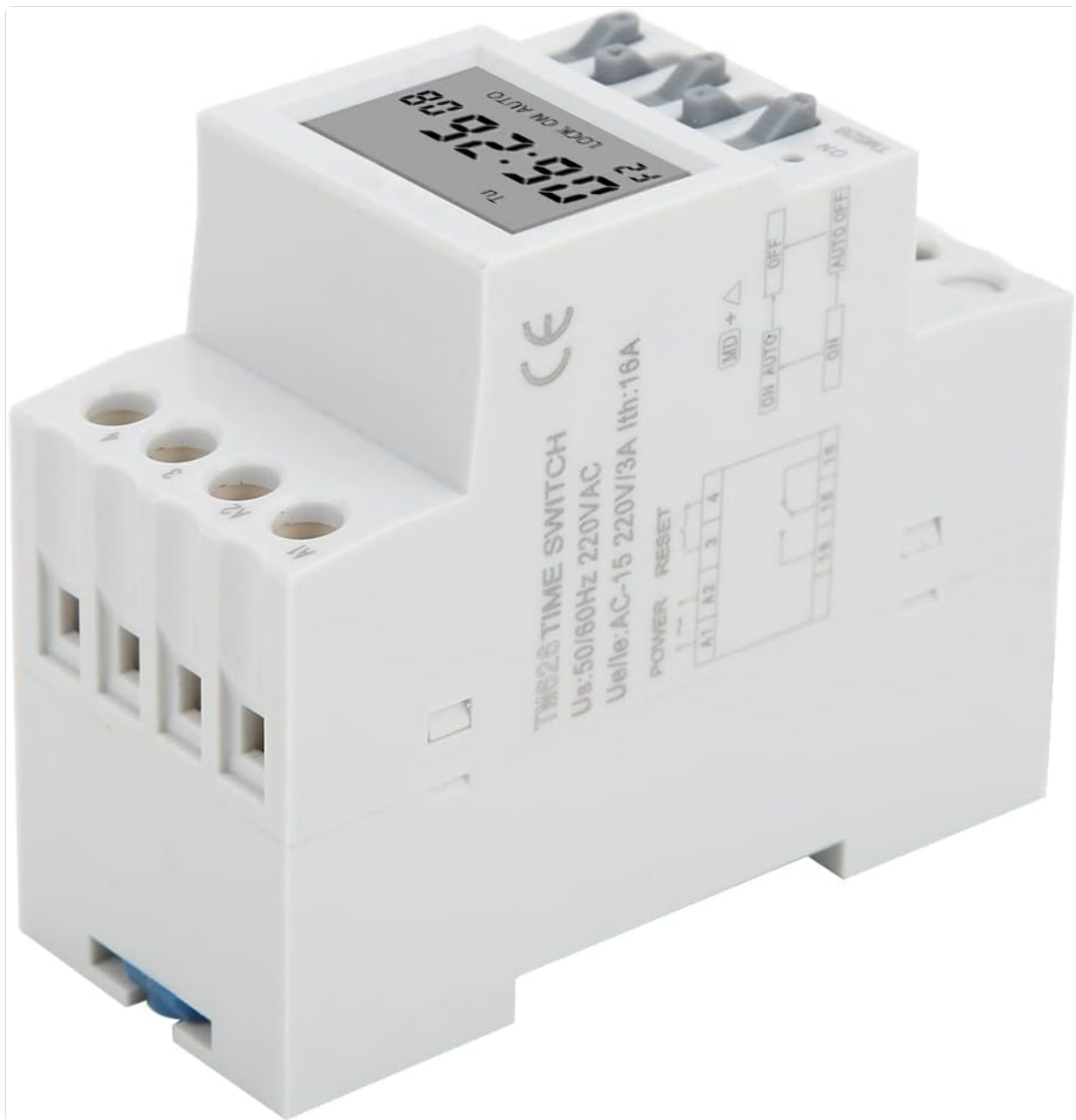
Image 5.1: Side view of the TM626 showing the wiring terminals and a simplified internal diagram. Terminals A1 and A2 are for power input (AC220V). Terminals 15, 16, 18 are for load output (15: Common, 16: Normally Closed, 18: Normally Open).
