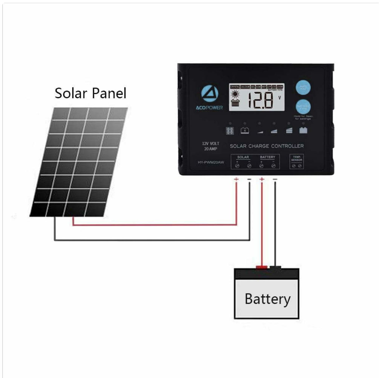
Figure 5.2: Wiring diagram showing the correct connection order: solar panel to controller, and controller to battery.
