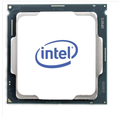
Figure 3.1: Top view of the Intel Xeon E-2236 Processor. This image shows the integrated heat spreader (IHS) with the Intel logo, and the orientation marks for proper socket alignment.
