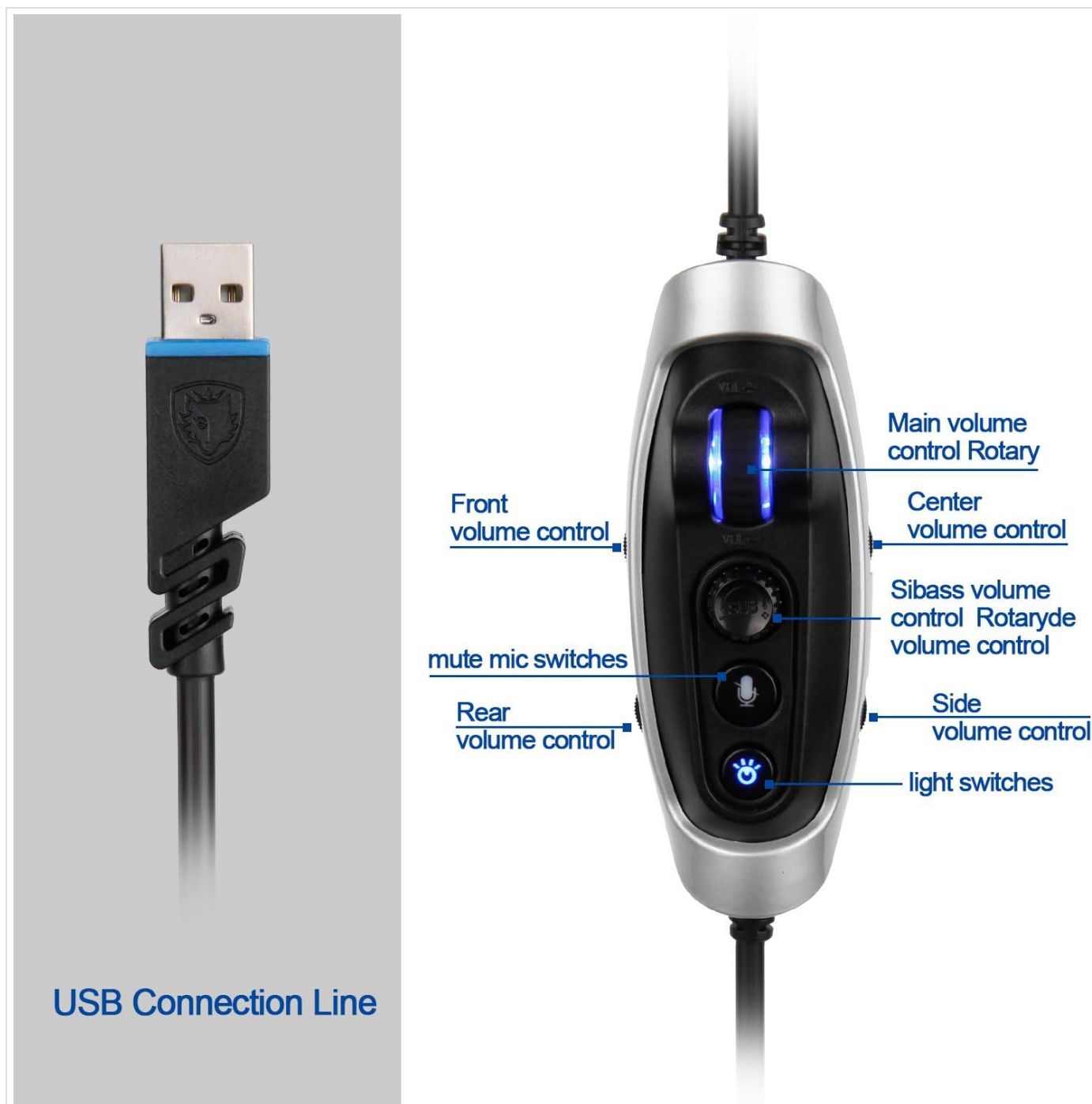
Figure 2: Detailed view of the inline control unit, indicating the Main Volume Control, Front Volume Control, Center Volume Control, Sibass Volume Control, Side Volume Control, Microphone Mute Switch, and Light Switches.
