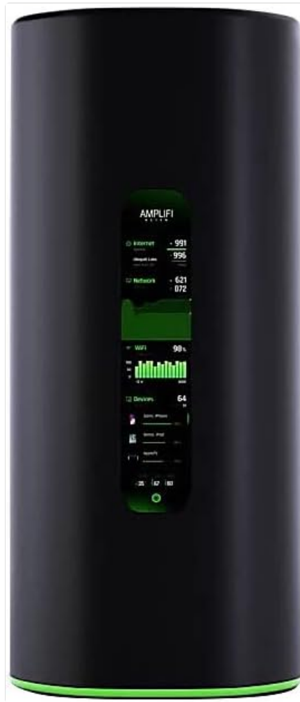
Figure 4.1: Close-up of the AmpliFi Alien Router's touchscreen, showing network performance metrics.
