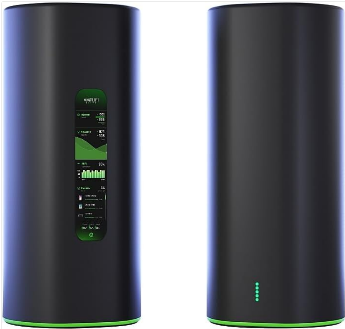
Figure 2.1: Front and back view of the AmpliFi Alien Router, highlighting the touchscreen display on the front.
