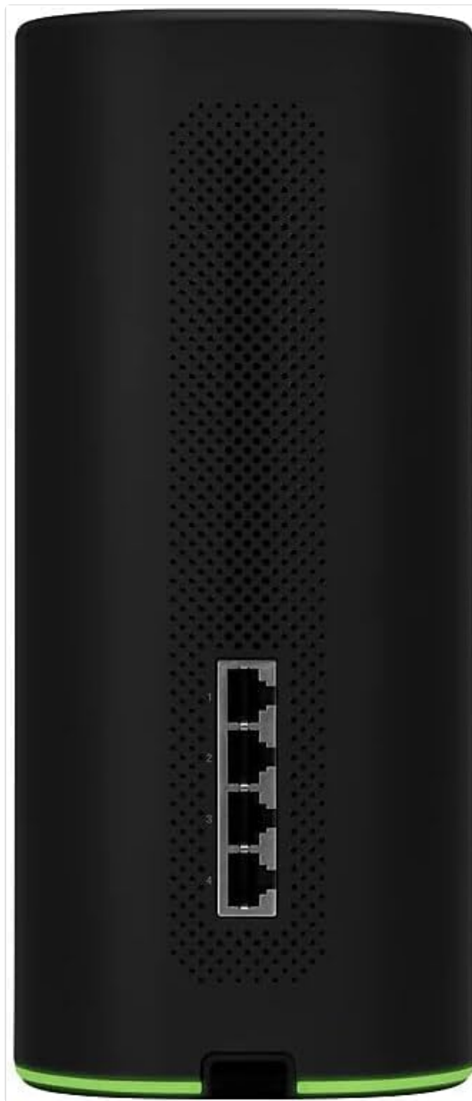
Figure 3.1: Rear view of the AmpliFi Alien Router, showing the four Gigabit Ethernet LAN ports and the WAN port.
