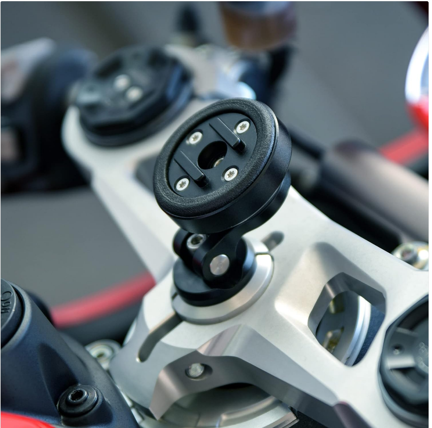
Figure 2: The SP Connect Anti Vibration Module installed on a motorcycle handlebar mount, viewed from a slightly elevated angle, showing its integration with the motorcycle's existing structure.
