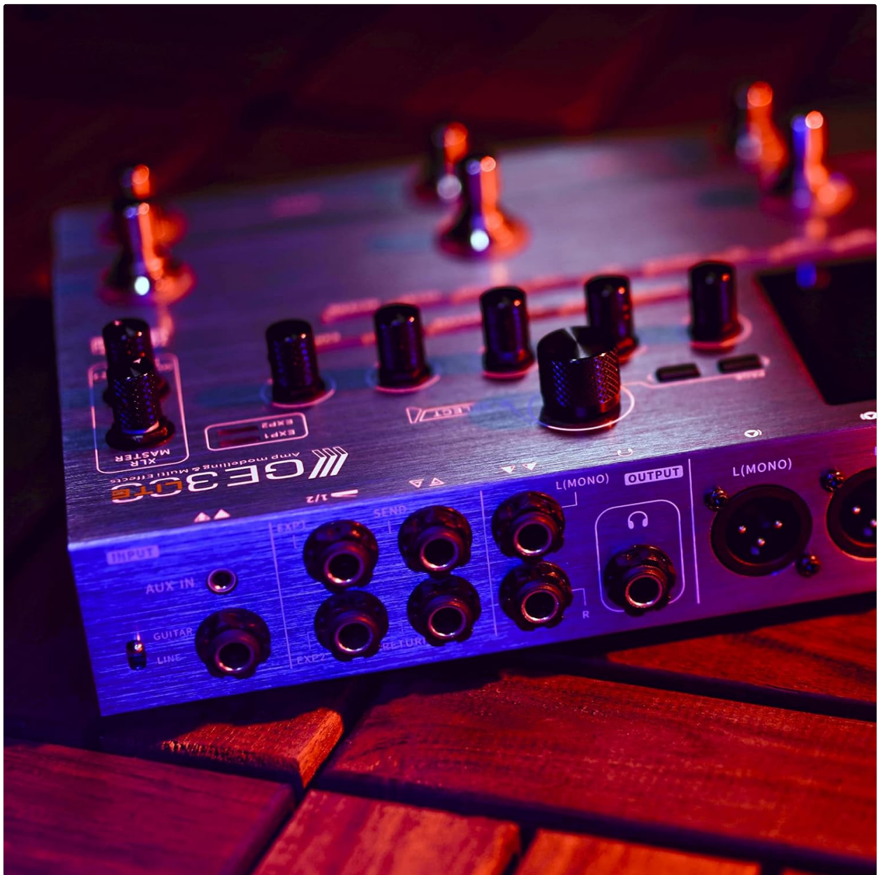
Figure 2: Rear view of the MOOER GE300 Lite, showing all input and output jacks.
