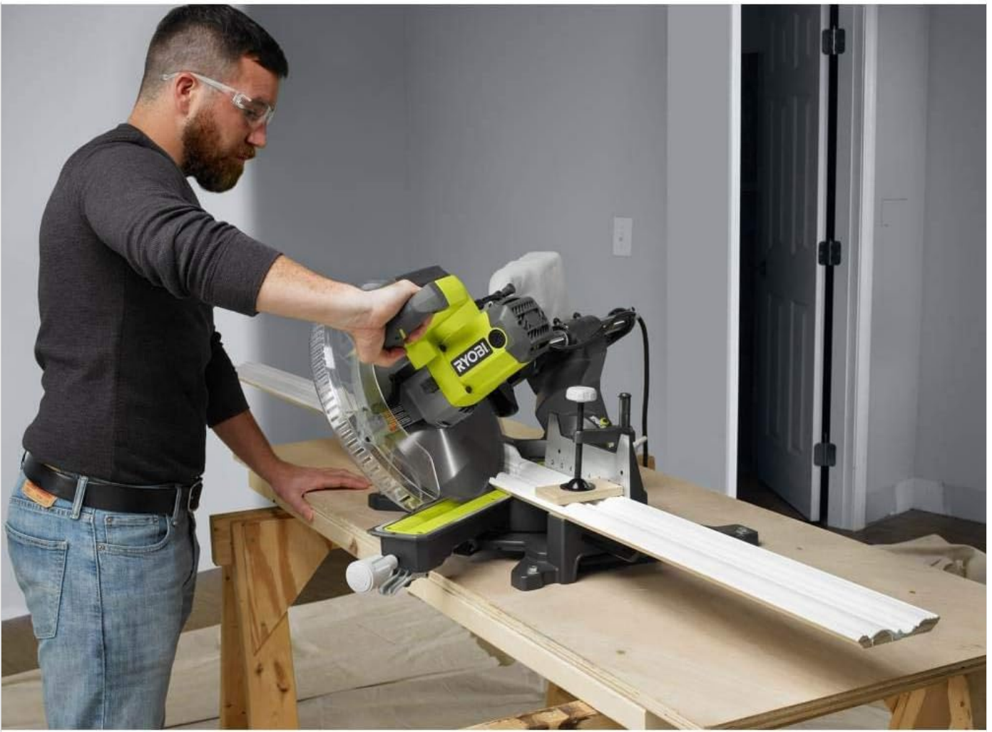
Figure 6: An operator making a precise cut on a piece of trim using the miter saw, demonstrating proper technique and safety.
