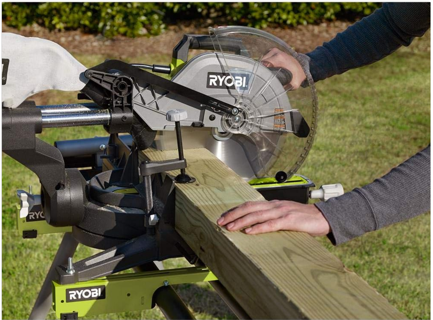
Figure 7: An operator cutting a larger piece of lumber, highlighting the use of the work clamp for stability.
