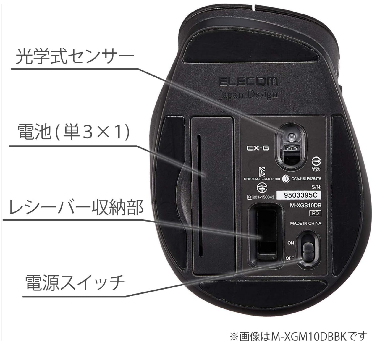
Image 2.2: Bottom view of the mouse, highlighting the optical sensor, battery compartment, receiver storage, and power switch.
