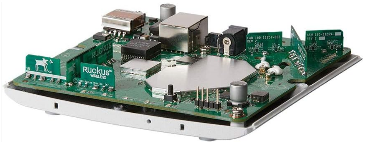
Figure 4.3: Internal view of the Ruckus R320 Access Point. This image shows the green circuit board with various electronic components, including chips, capacitors, and connectors, illustrating the device's internal hardware architecture.
