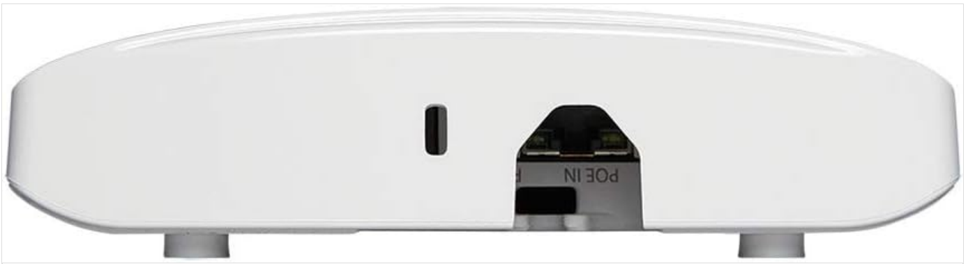
Figure 4.1: Side view of the Ruckus R320 Access Point. This image highlights the recessed Power over Ethernet (PoE) input port, labeled "POEIN", and a small indicator light slot on the side of the white casing.
