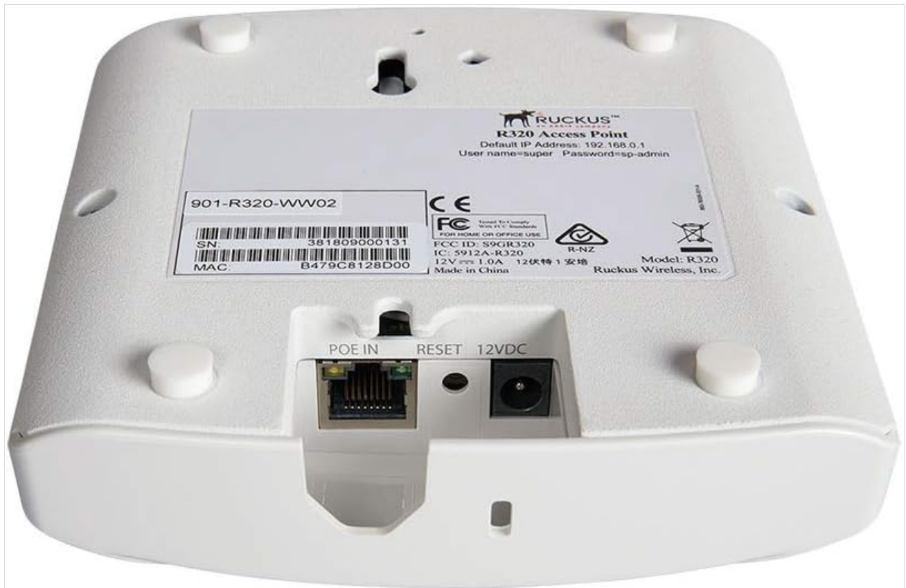
Figure 4.2: Bottom view of the Ruckus R320 Access Point. This image displays the product label with model information (R320), default IP address (192.168.0.1), username (super), and password (sp-admin). It also clearly shows the "POEIN" Ethernet port, a "RESET" button, and a "12VDC" power input port.
