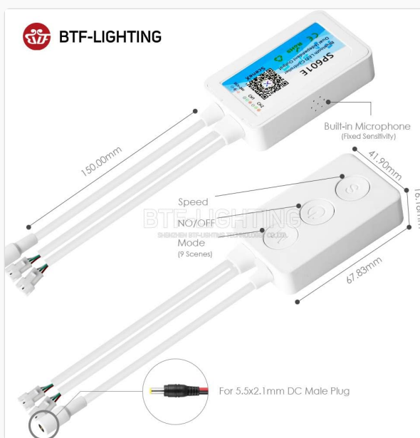
Figure 1: SP601E Controller Layout. This image displays the BTF-LIGHTING SP601E controller with its dimensions (150.00mm cable length, 41.90mm width, 16.18mm height) and button functions: Speed (S), ON/OFF (Power), and Mode (M). It also shows the 5.5x2.1mm DC male plug connection.
