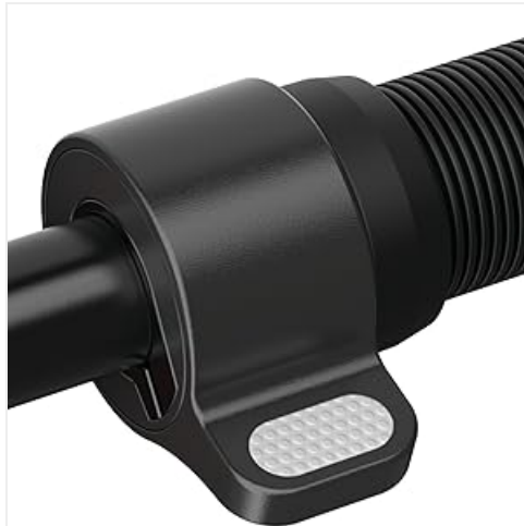
Figure 4.2: Close-up of the thumb-activated throttle control.
