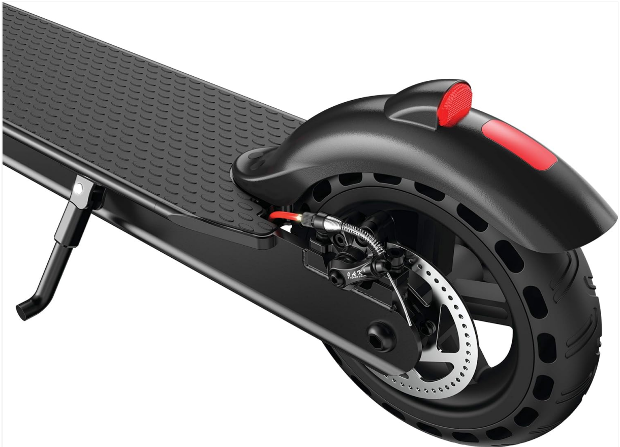
Figure 4.4: Rear wheel with disc brake and brake-activated taillight.
