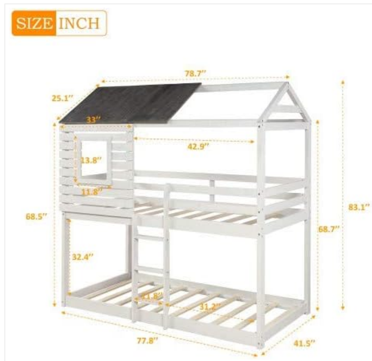
Image 3.1: A diagram illustrating the precise measurements of the bunk bed, including overall length (77.8"), width (41"), height (83.1"), and specific dimensions for the roof, window, and bunk heights. This image is essential for understanding the bed's footprint and clearances.
