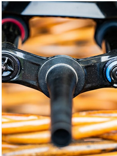
Figure 2: Top cap showing the air valve for pressure adjustment.
