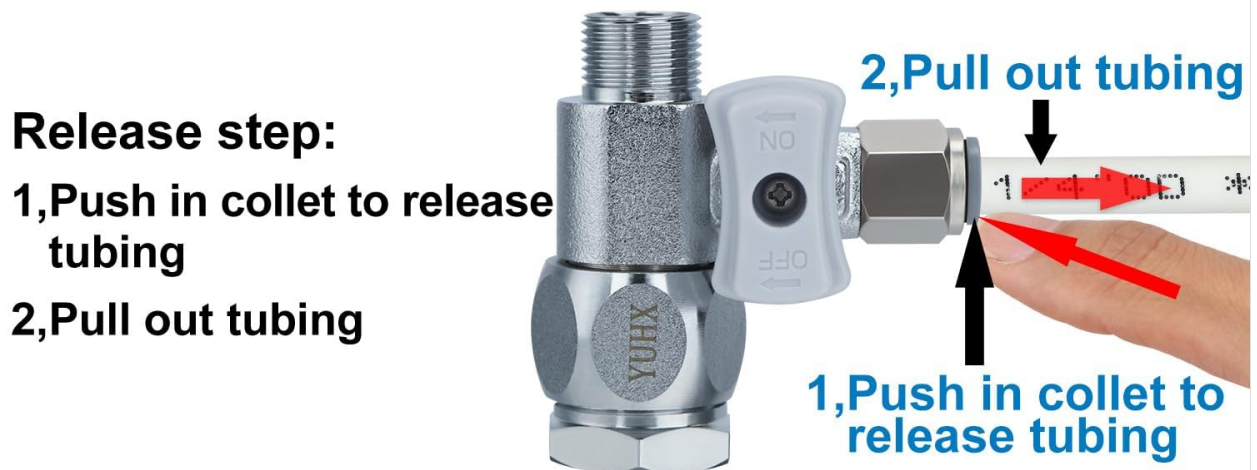
Figure 3: Push-to-connect installation and release method.
